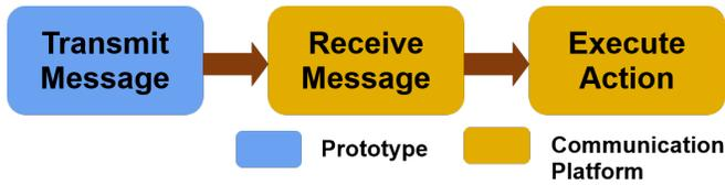
Fig. 1. Communication model using a WLAN between the smartwatch prototype and the communication platform.
